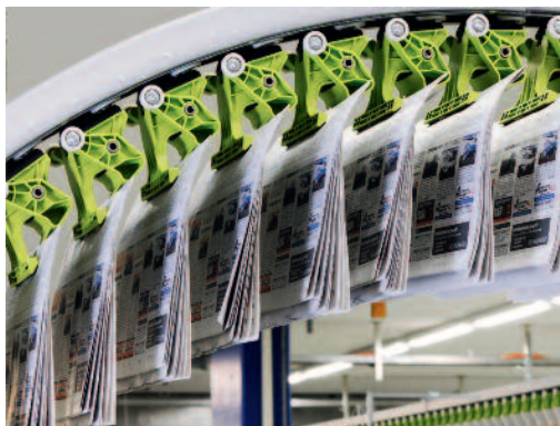
The chains and clamps of the High Performance Conveyor system are made of plastic.
