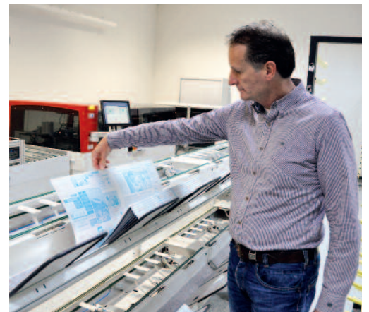
Hans Daniels, general plant manager at BDU Print shows the double-spread plates for the new KBA Commander CT
