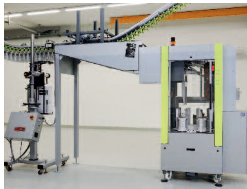
The HPS concept is based on Multi-Stack technology with servo drives throughout.
